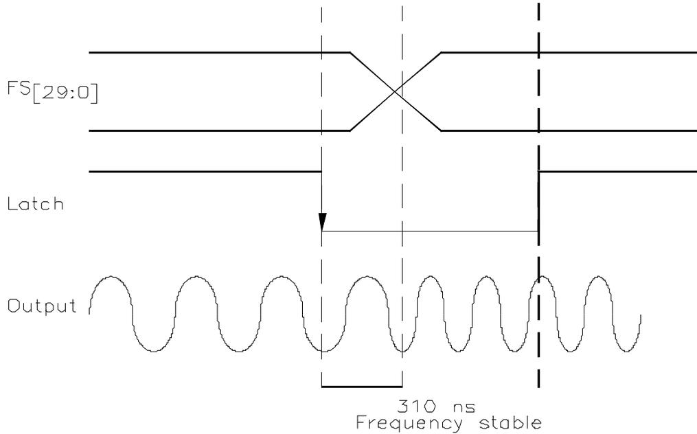
To generate a frequency chirp, set the starting frequency as above and then apply the delta word to the FS input. A falling edge on DLATCH will then load the delta frequency word and initiate the chirp. The chirp will stop and output will return to starting value on a rising edge.
